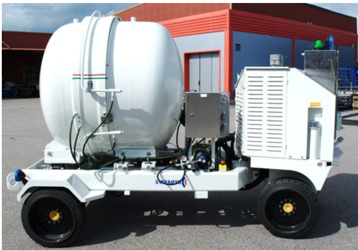
Fjärrstyrd bombvagn./Mobile explosion containment vessel, MECV.
